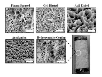
Fig.1Surface topography of implants undergoing different types of treatments
